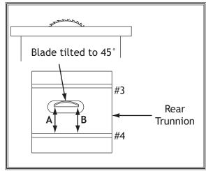
**Figure 99.** Locations of the rear trunnion shims.
